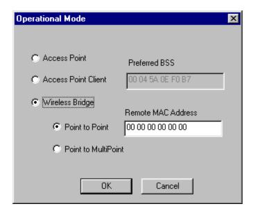
This will bring up the **Operational Mode** window. Within this window are all the modes in which the Access Point can communicate.
